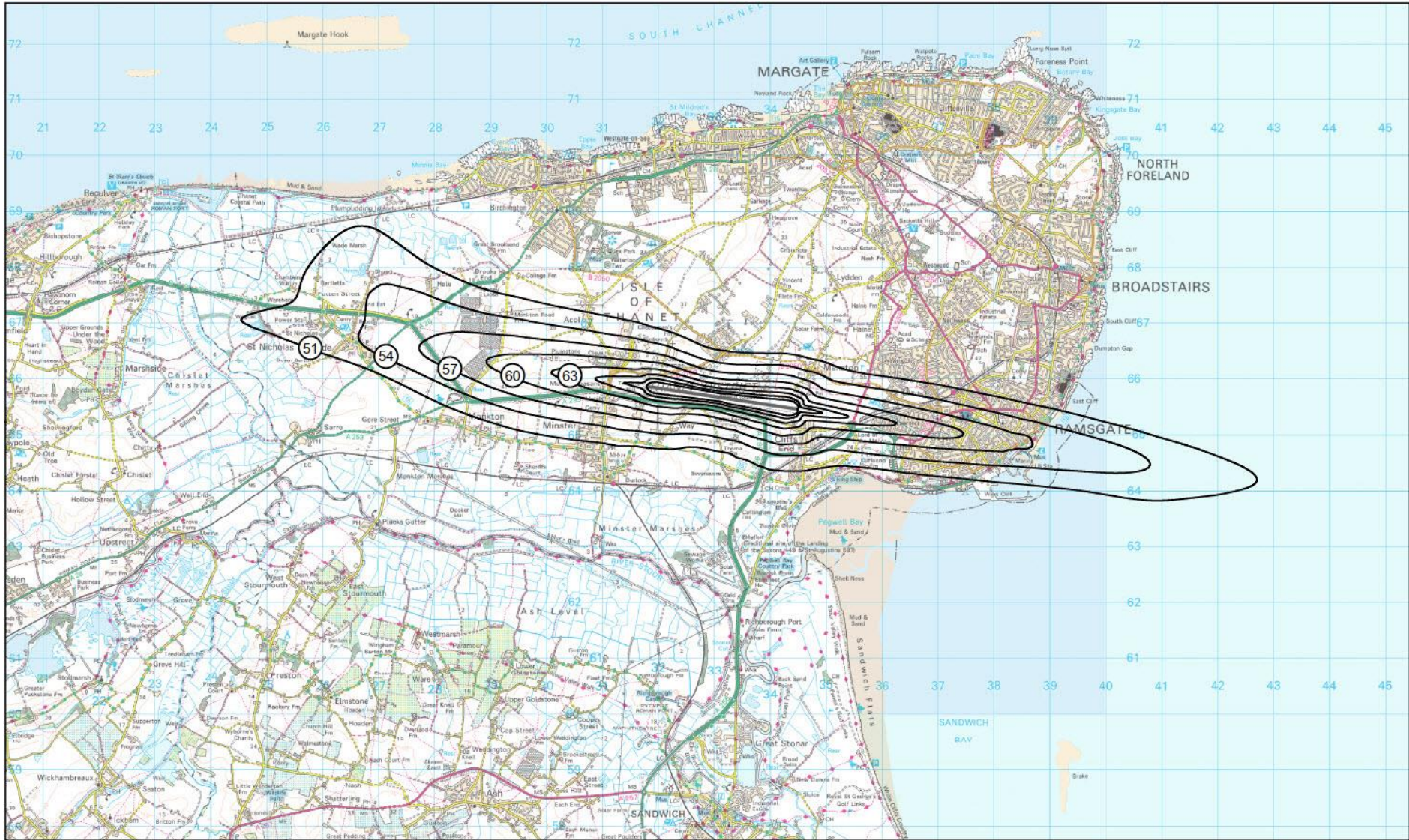
MANSTON AIRPORT 'NNF' Fleet Mix - Forecast Average Day LAeq,16hr 51-72 dB(A) Contours Runway Modal Split 70% W / 30% E
