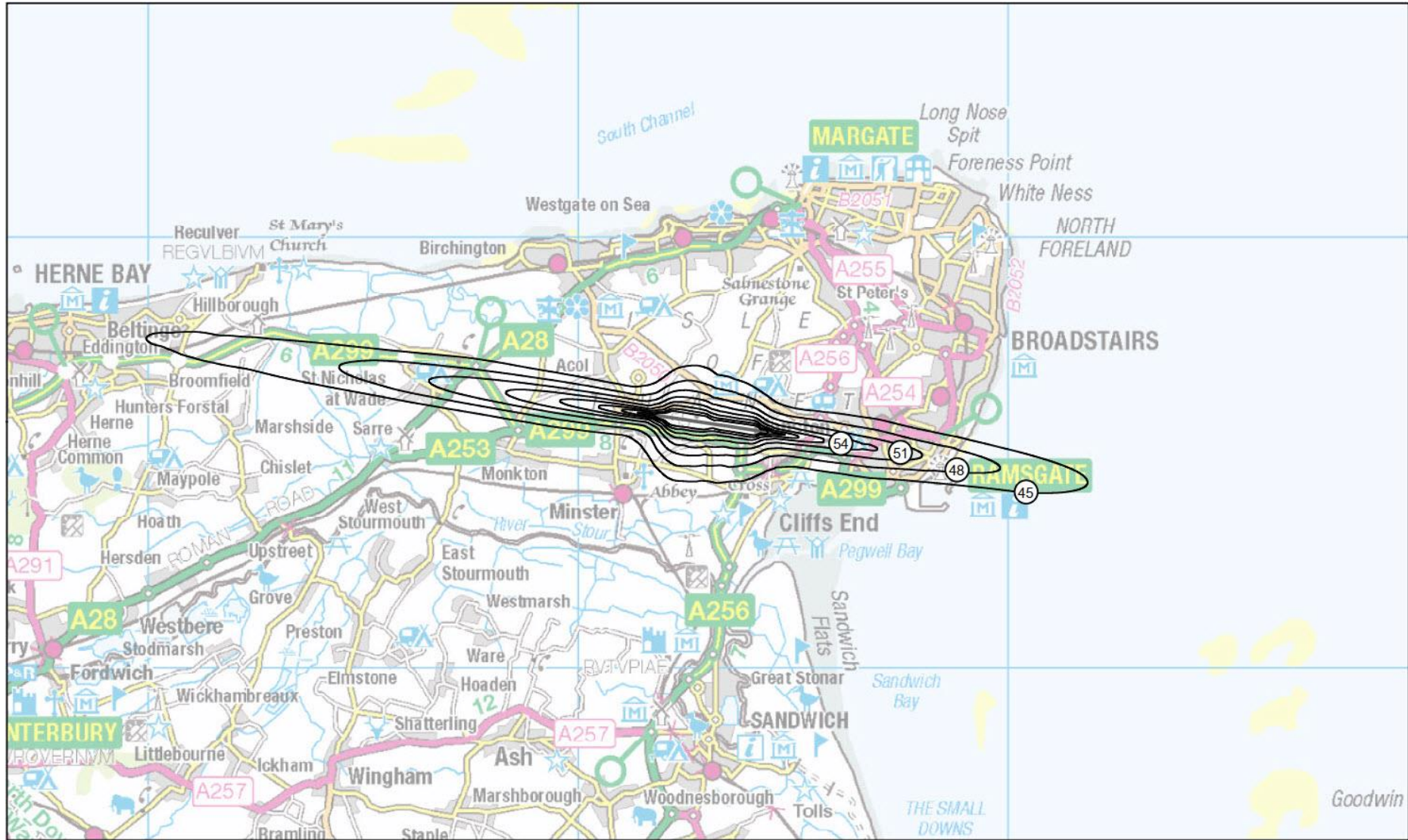
MANSTON AIRPORT 'NNF' Fleet Mix - Forecast Average Night L_{Aeq,8hr} 45-66 dB(A) Contours Runway Modal Split 30% W / 70% E
