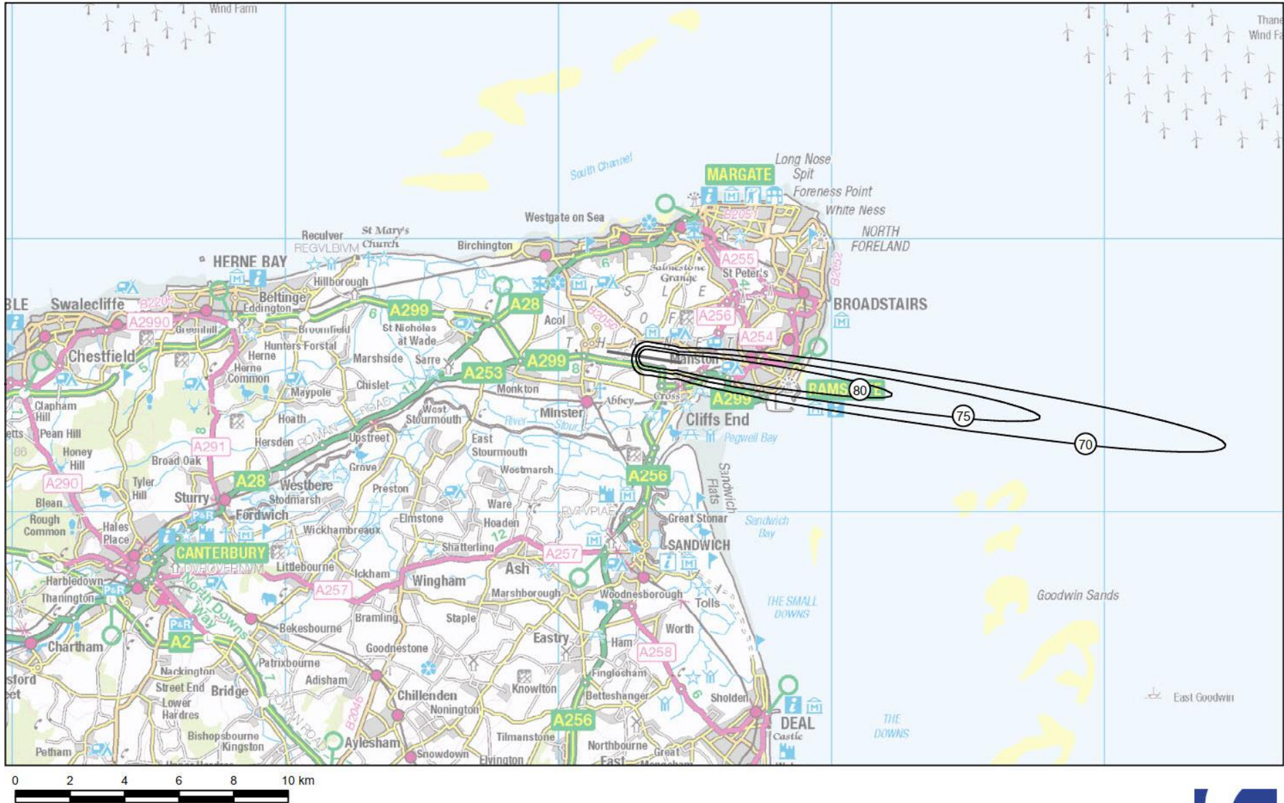
MANSTON AIRPORT B744G (Boeing 747-400 with GE CF6 engines) L Amax 70-80 dB(A) Footprints - RWY28 Arrival
