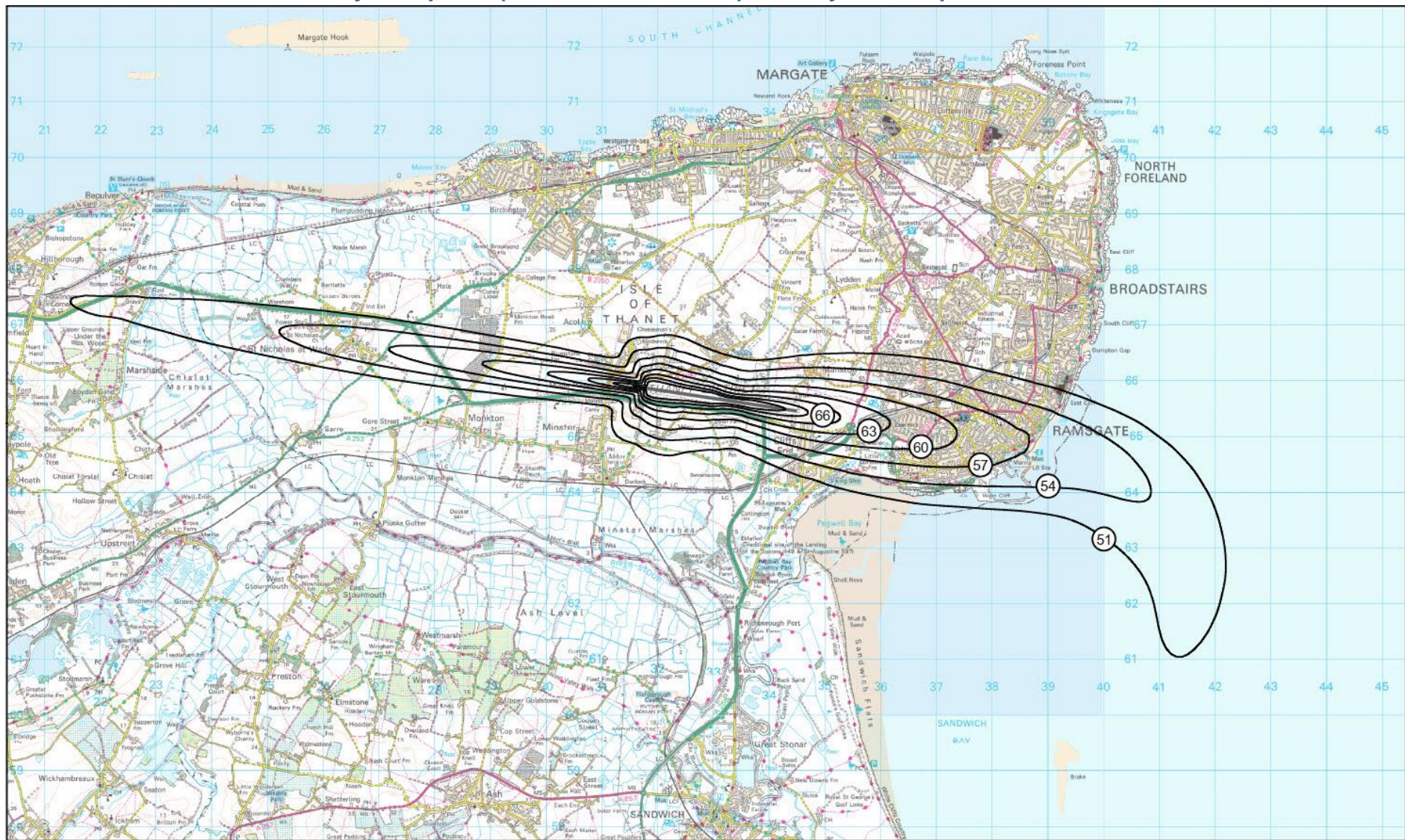
MANSTON AIRPORT 'NNF' Fleet Mix - Forecast Average Day LAeq,16hr 51-72 dB(A) Contours Runway Modal Split 100% E
