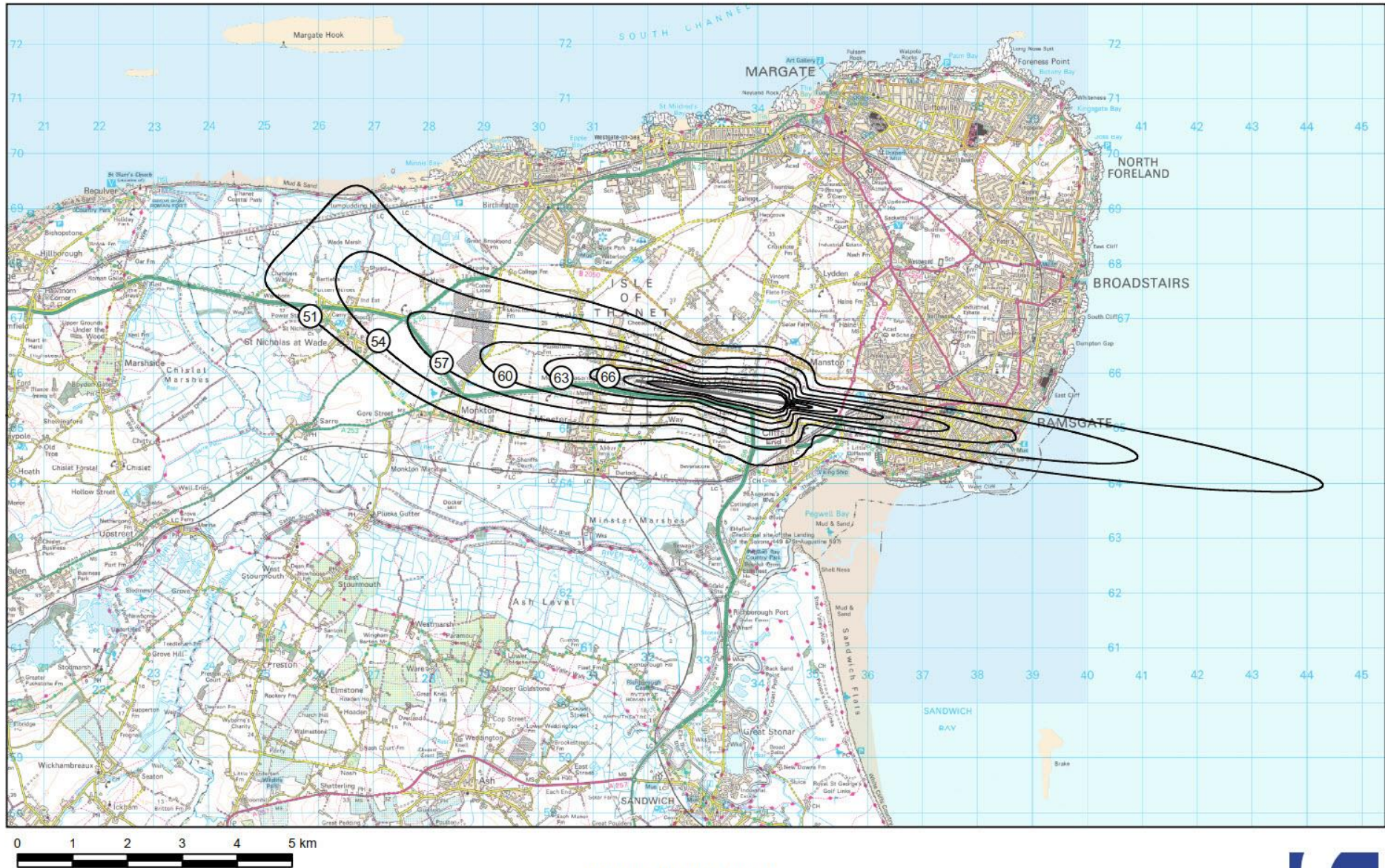
MANSTON AIRPORT 'NNF' Fleet Mix - Forecast Average Day L_{Aeq,16hr} 51-72 dB(A) Contours Runway Modal Split 100% W
