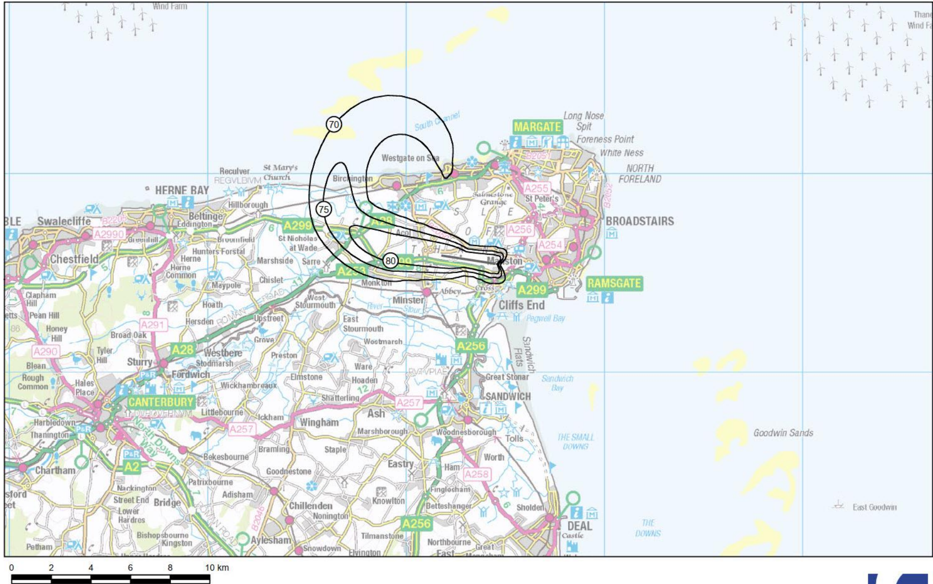
MANSTON AIRPORT B744G (Boeing 747-400 with GE CF6 engines) L Amax 70-80 dB(A) Footprints - RWY28 Departure Route 1
